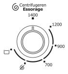
Turn the Spin selector to change the spin speed, if you want your laundry to be spun at a speed different from the one proposed by the washing machine.
